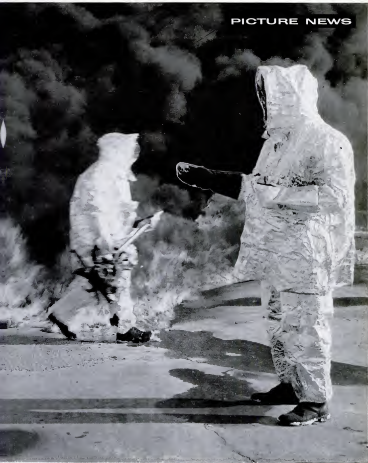
GIs wear paper suits to fight fires. Carrying lightweight hose and piping right to the edge of a fire, these soldiers are protected by the Army's new aluminized kraft-paper fire-fighting garb. Wearing the expendable suits over uniforms, troopers were able to stand within two feet of flames for two to three minutes without discomfort although exposed parts of helmet liners were blistered. They made quick work of the fire.
